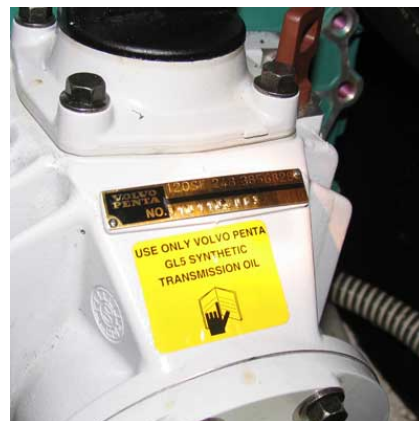
Saildrive 120S E: Use only Volvo Penta GL5 Synthetic transmission oil.
