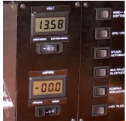
De startaccu is vol, laadstroom nul.
